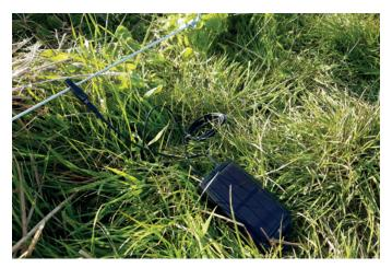
Fig. 5. Fence monitor saving voltage data (Photo: Timo Nolte).
