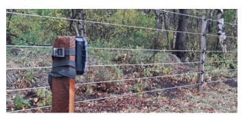
Fig. 6. Typical set-up of a camera trap to monitor wildlife in the vicinity of a wolf-deterrent permanent electric fence (Photo: Timo Nolte).
