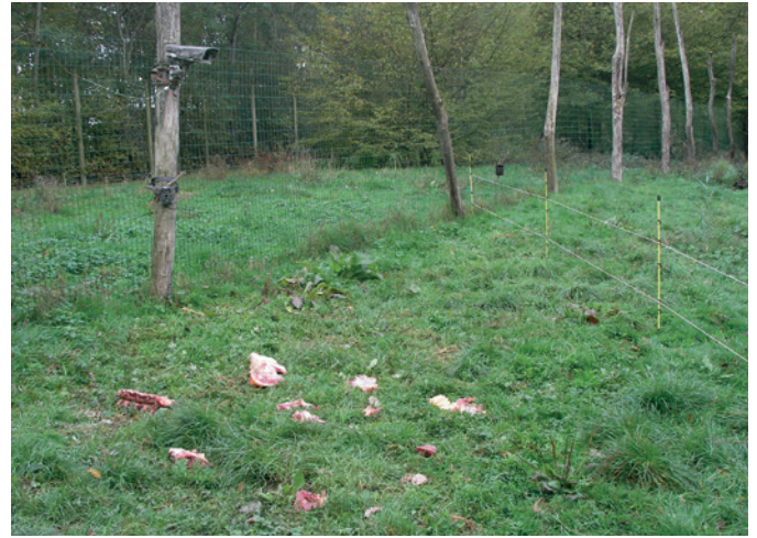
Fig. 3. Meat left during an experiment in the grey wolf enclosure. In this case, a two-wire fence was tested. A thermal camera and two remote cameras can be seen, fixed on wooden poles and facing towards the fence or meat.
