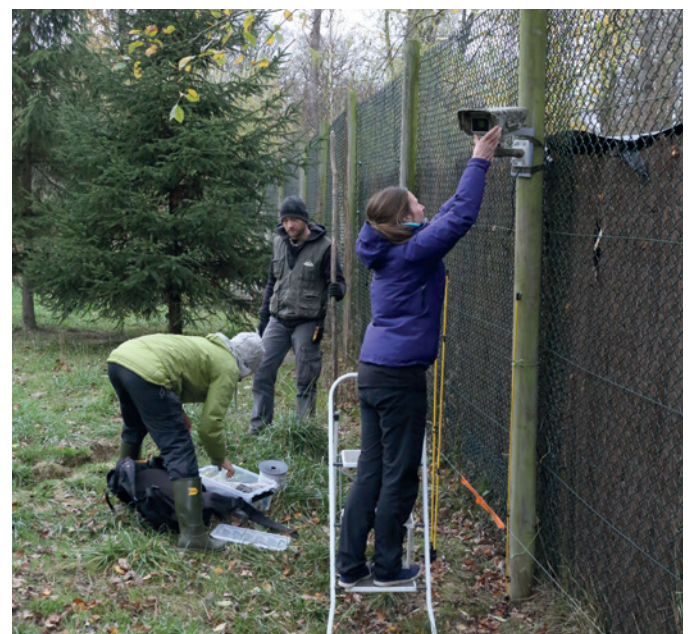
Fig. 2. Installation of the camera equipment: remote camera (Bushnell, above) and thermal camera (AXIS Q1921-E, below).
