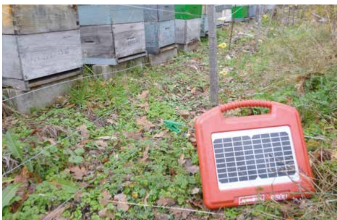
Photovoltaic energizer used during the essay. Photo: J.M. Seijas.
