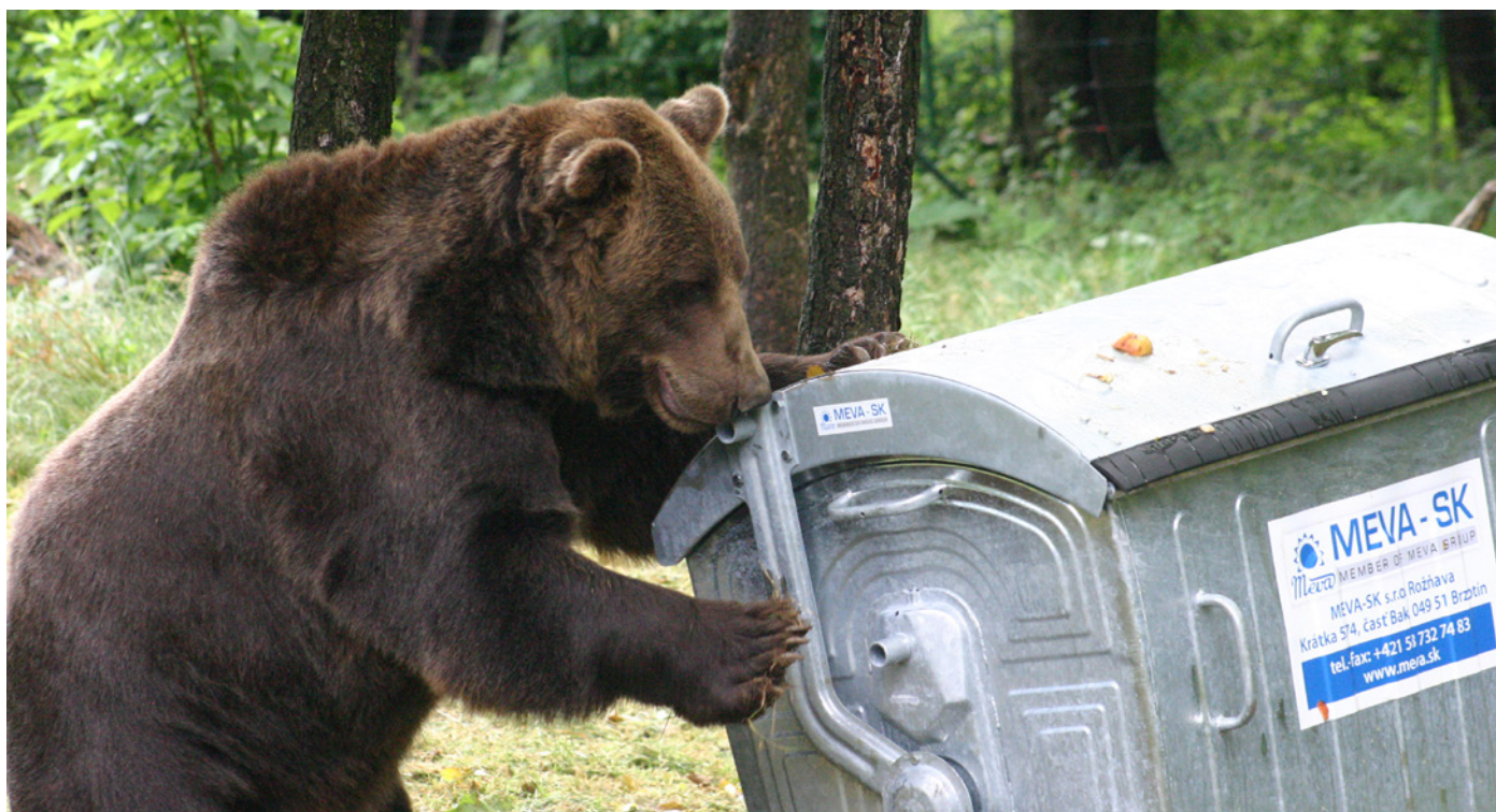
Fig. 8. A modified and reinforced refuse container undergoing testing (Photo: Robin Rigg).
